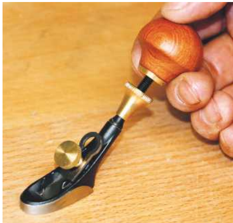
▲ By unscrewing the top part of the handle the length can be extended
